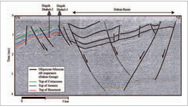
Figure 7 Regional seismic profile crossing Dagah Shabel and Daban basin illustrating a graben structure of the Oligocene-Miocene units and the overall structural style of the area.
